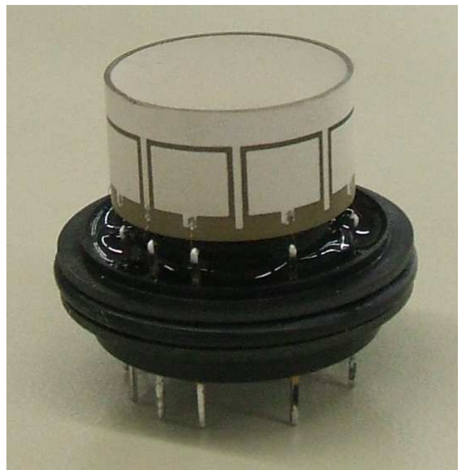
Fig. 3. Vibrating Structure Gyro. This piezoelectric gyro was a production item made by BAE Systems.
