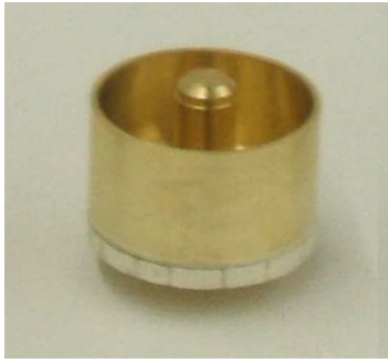
Fig. 22. A cup gyro with a hybrid structure. The electrode interface utilizes a piezoceramic ring bonded to the bottom of a metal cup.
