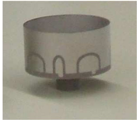
Fig. 14. An example of skewed electrode placement. The drive electrodes are skewed by 6° and the smaller node electrodes are skewed by 2°.
